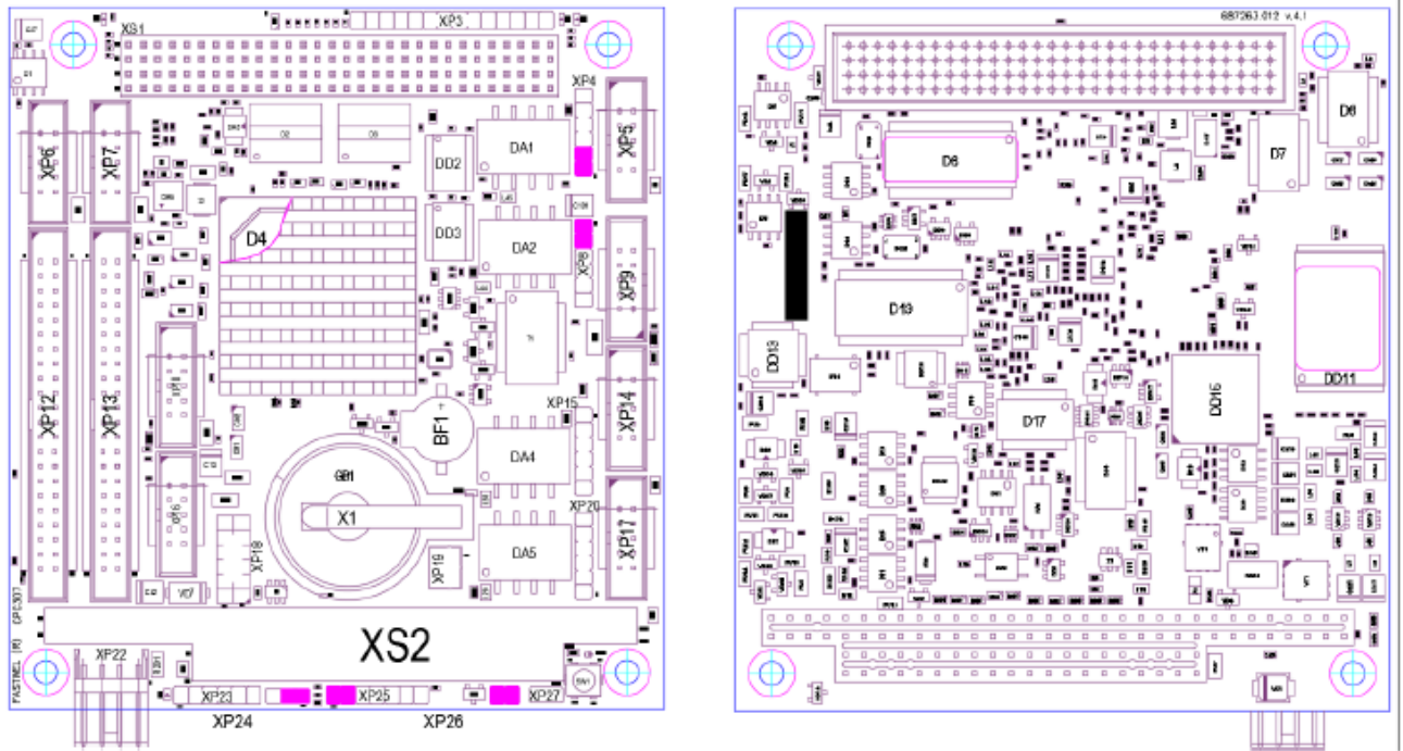
Figure 4.3 b) Location of connectors and main components on the TOP and BOTTOM sides of the CPC307-02, CPC307-05 versions (relevant to CPC307 v.4.x)
